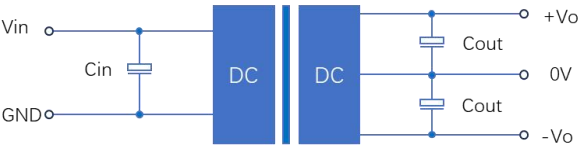
Figure 1: Application circuit 图1：应用电路
