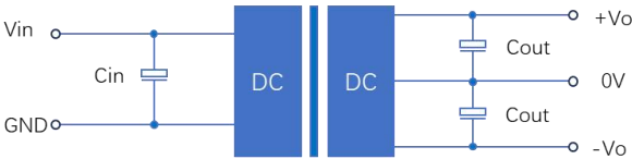
Figure 1: Application circuit 图1：应用电路
