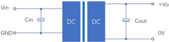
Figure 1: Application circuit 图1：应用电路
