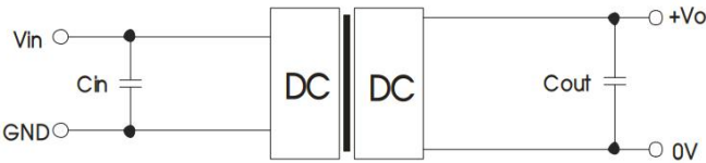
Figure 1: Application circuit 图1：应用电路
